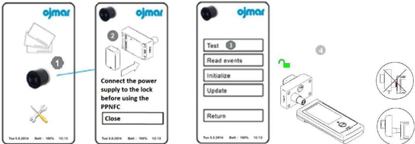
**TEST:** Performs a test on the lock and displays the results on the screen. To do so:
